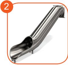
Tube slide made of stainless steel AISI 304. The metal sheet is 2 mm thick and the end section is finished with a band made of pipe 33,7 mm. The surface is polished.
