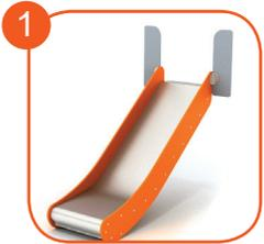
Slides made of stainless steel AISI 304. Metal sheet with a thickness of 2 mm formed in a CNC technique. Side panels made of HDPE polyethylene 15 mm, in the highest quality and totally damp-proof and resistant to UV.
