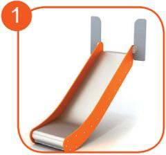
Slides made of stainless steel AISI 304. Metal sheet with a thickness of 2 mm formed in a CNC technique. Side panels made of HDPE polyethylene 15 mm, in the highest quality and totally damp-proof and resistant to UV.
